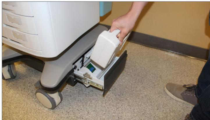
5. Push the battery down to reposition the receptacle so the battery box can be closed.
