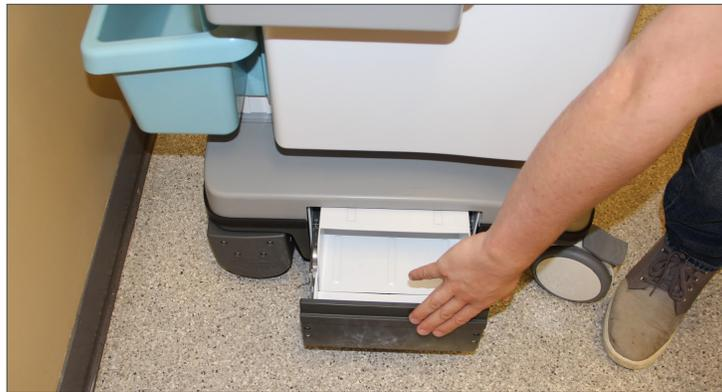
3. The battery receptacle will be in a horizontal position by default. Reach down into the battery box and push the back of the receptacle down, to properly orient the compartment for battery placement.
